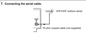
If you connect a VCR, connect the aerial output jack of your VCR and the aerial jack on the TV with aerial cable. Then connect the output jacks of your VCR and the VIDEO-1 input jacks of the TV with the video cable (or S-VIDEO cable if available) and audio cables. For details, see the manual of your VCR.
